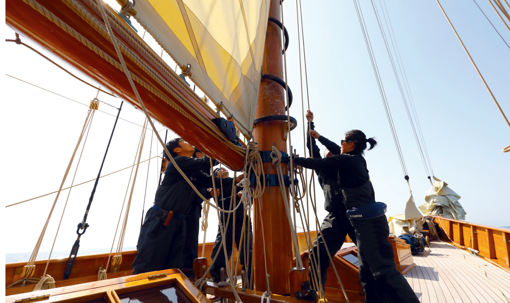
All new masts and spars for the gaff rig are in Douglas fir
