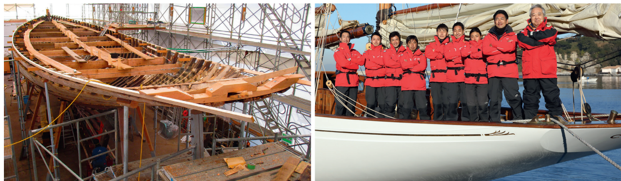
Left: hull was stripped back to the bare bones. Right: Mr Watanabe (right) and Cynara's Japanese crew
